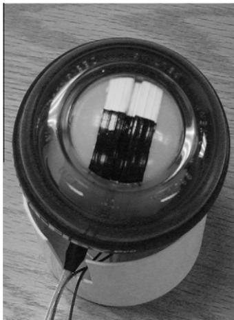
**Fig. 1.** The top view of a roller ball that was used in the experiments. The opening on the outer shell reveals the inner top which spins when applying torque from the outer shell. The equator of the inner top was painted half white and half black in order for the optic fiber to detect the different reflective light.
